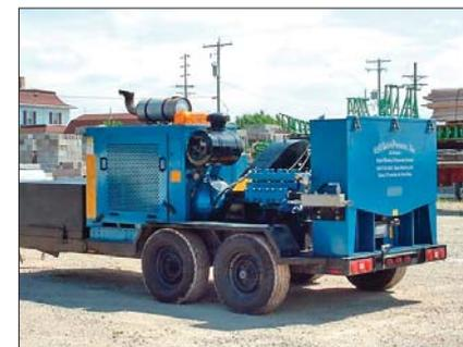
This NLB hydroblaster, capable of up to 20,000 psi or 60 gpm, is one of five hydroblasters in the fleet of H<sub>2</sub>O Underpressure, which started with one blaster just five years ago.
